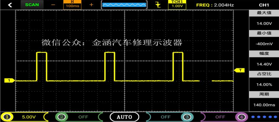
Oxygen sensor heating signal
