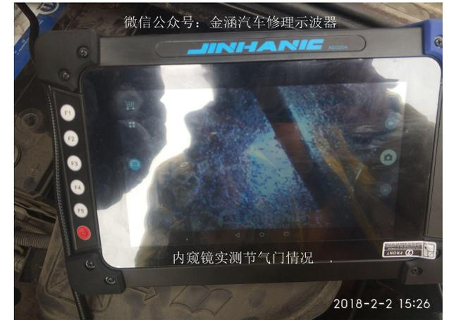
Endoscope measured throttle condition
