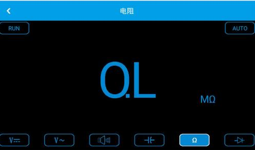
② Connect the measurement probe to the two ends of the resistance to be measured. The display value can be read out. If needed, the range can also be manually set.
