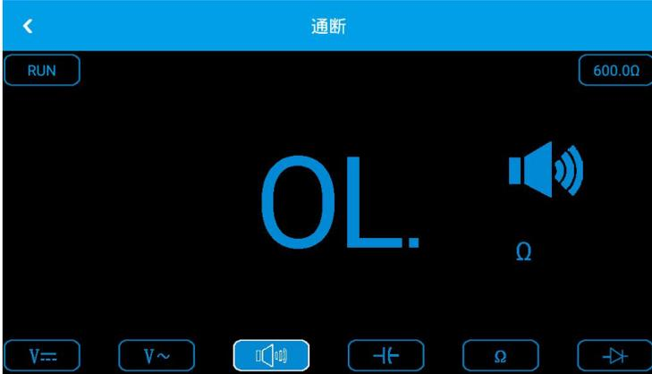
② Connect the test leads to the ends of the diode or line to be tested and read the readings. (Measured diode reading is diode turn-on voltage drop)
