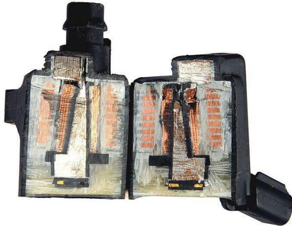
Cross section of ignition coil (inside secondary coil, outside primary coil)
