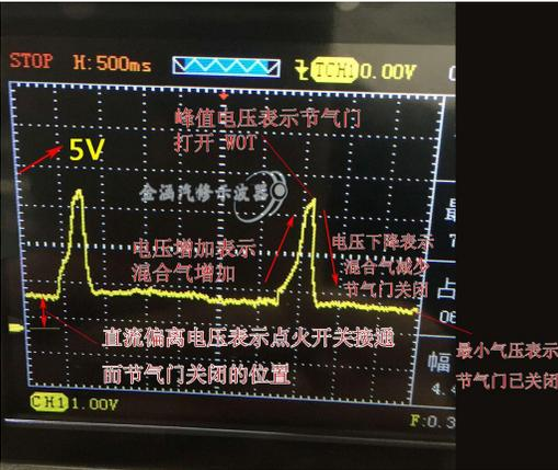
Now the throttle position sensor has two signals. The maximum voltage of the two signal lines together is 5v. The right figure shows the old cable-type throttle position sensor waveform.
