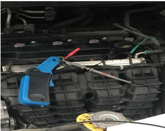
Figure 7 : Usage of current clamp.
