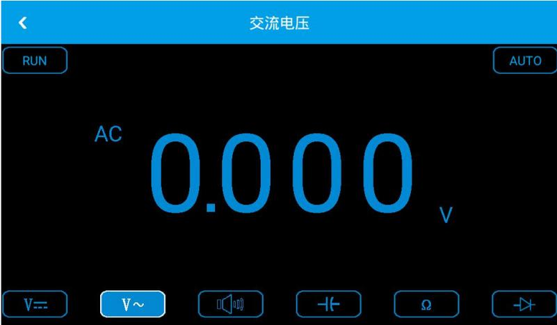
④ Connect the test pen to the voltage to be measured or the power supply to read out the displayed value. At the same time, the polarity of the end of the red lead can also be seen by the positive and negative values displayed on the LCD. (The polarity is not displayed when the AC voltage is measured.) This instrument defaults to the "Auto" range. If you need to manually set the range, you can change the range by clicking the "AUTO" icon and then perform the measurement.
